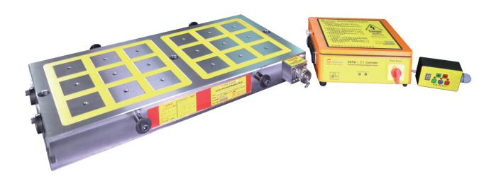
Pole 70X70 mm, Flux Line 40 mm, Magnetic Force 2800±5% kgf/4 Poles
