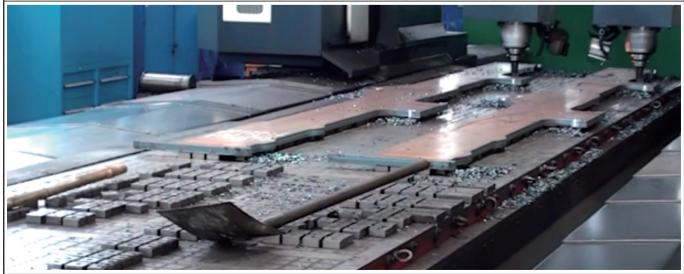
Used on Double Column Machining Center for machining big & multi-medium workpiece 5 sides machining.
